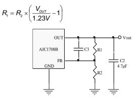
Fig. 2 AIC1708B with External Resistor Divider
