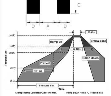
**Solder Pad Layouts** В С Part number (mm) (mm) (mm) 0.80 0.60 0.80 LP-TSML035
