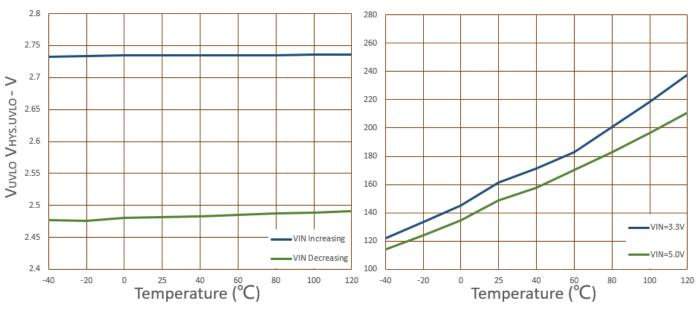
Undervoltage Lockout vs Free-Air Temperature
