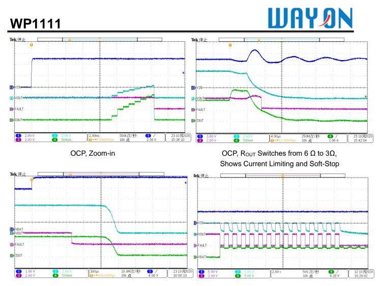
BAT-OVP, VVBAT Steps from 3.5 V to 4.4 V, Shows tDGL(BAT-OVP) and Soft-Stop
