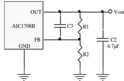
Fig. 2 AIC1708B with External Resistor Divider
