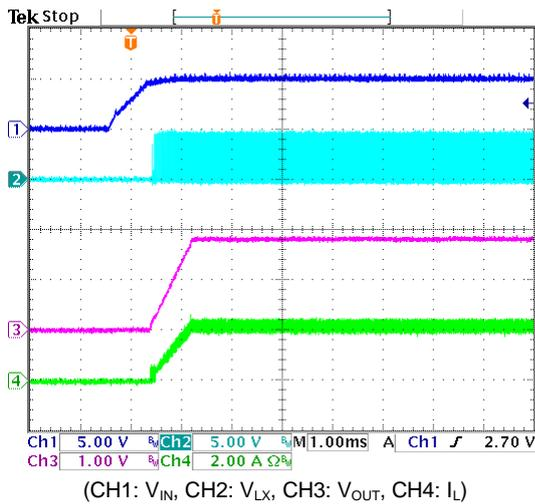
Fig. 10 V<sub>IN</sub> Power On (V<sub>IN</sub>=5V, V<sub>OUT</sub>=1.8V, I<sub>OUT</sub>=2A)
