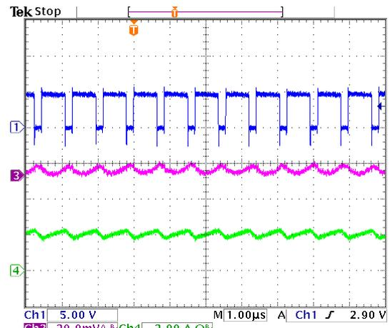
(CH1:  $V_{LX}$ , CH3:  $V_{OUT(ac)}$ , CH4:  $I_L$ )
