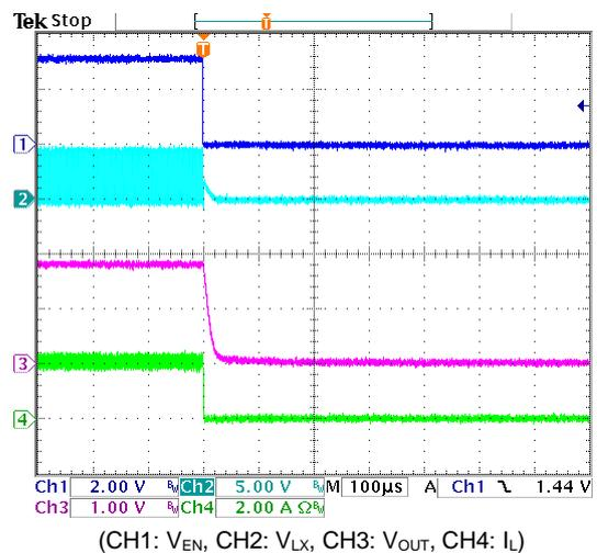
Fig. 13 Enable Off (V<sub>IN</sub>=5V, V<sub>OUT</sub>=1.8V, I<sub>OUT</sub>=2A)
