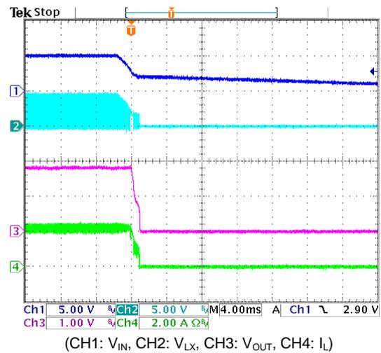
Fig. 11 V<sub>IN</sub> Power Off (V<sub>IN</sub>=5V, V<sub>OUT</sub>=1.8V, I<sub>OUT</sub>=2A)
