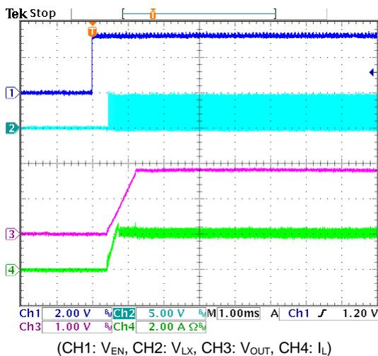
Fig. 12 Enable On (V<sub>IN</sub>=5V, V<sub>OUT</sub>=1.8V, I<sub>OUT</sub>=2A)
