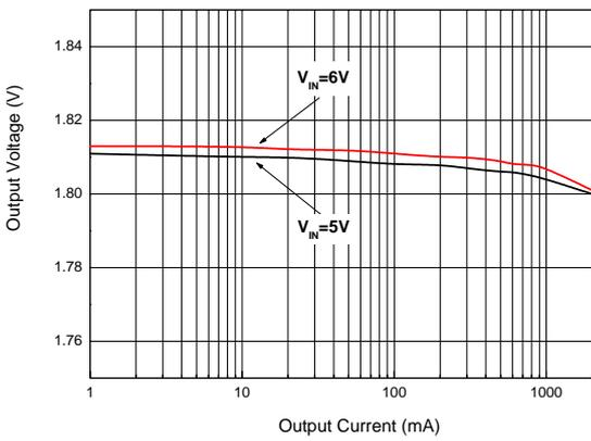
Fig. 4 Output Voltage vs. Output Current ( $V_{OUT}=1.8V$ )
