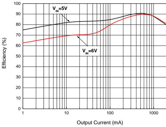
Fig. 2 Efficiency vs. Output Current ( $V_{OUT}=1.8V$ )
