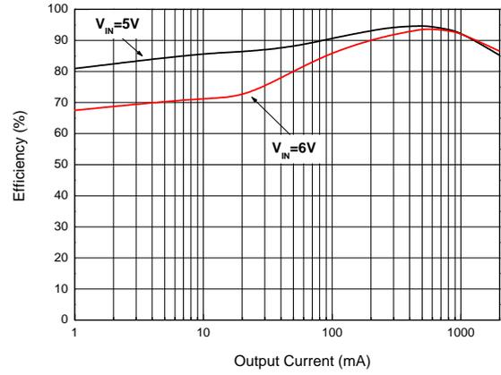
Fig. 3 Efficiency vs. Output Current ( $V_{OUT}=3.3V$ )
