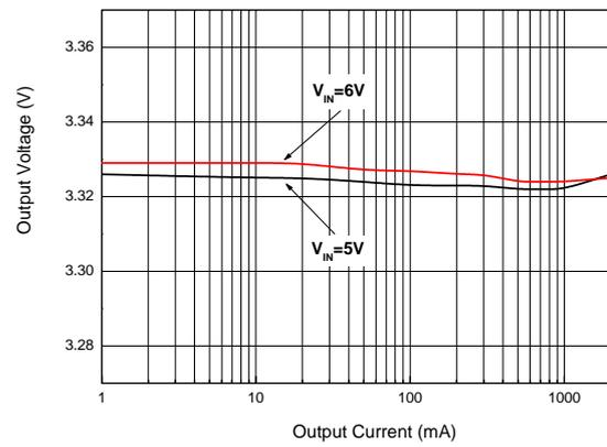
Fig. 5 Output Voltage vs. Output Current ( $V_{OUT}=3.3V$ )
