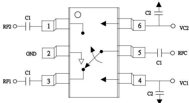
DC blocking capacitors C1 are required on all RF ports.
